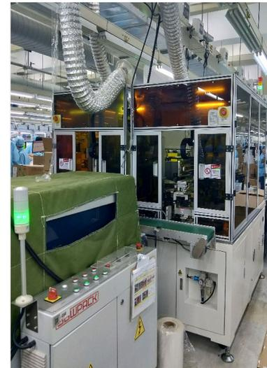
Power consumption of first-generation angle cutters: 12KW
